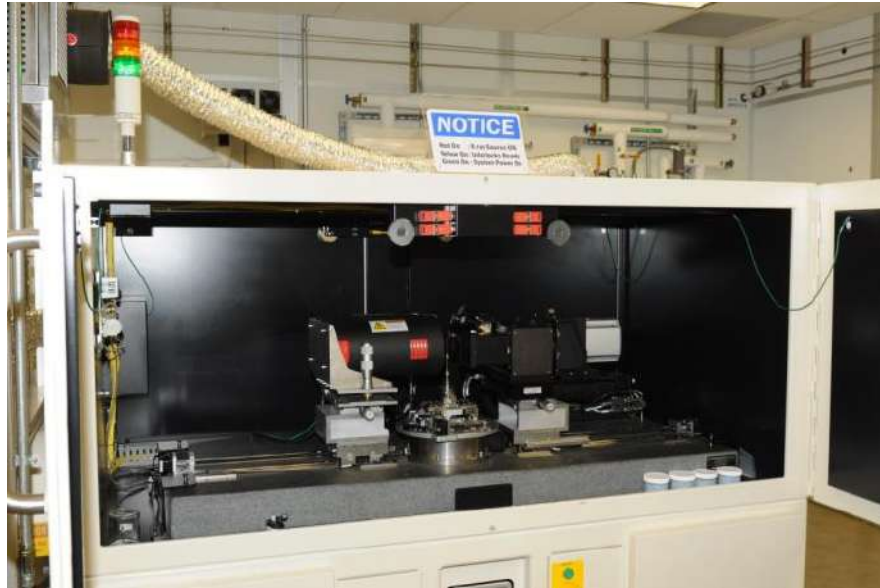
Figure 8-12. The micro-CT scanner at NETL. Source is on the left, rotating stage is the pedestal in the center, and detector is on the right.
