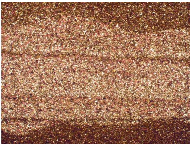
Figure 5-12. Thin section photomicrograph from the Richman Farms well showing ripple cross lamination overlying scour surface from Richman Farms well.
