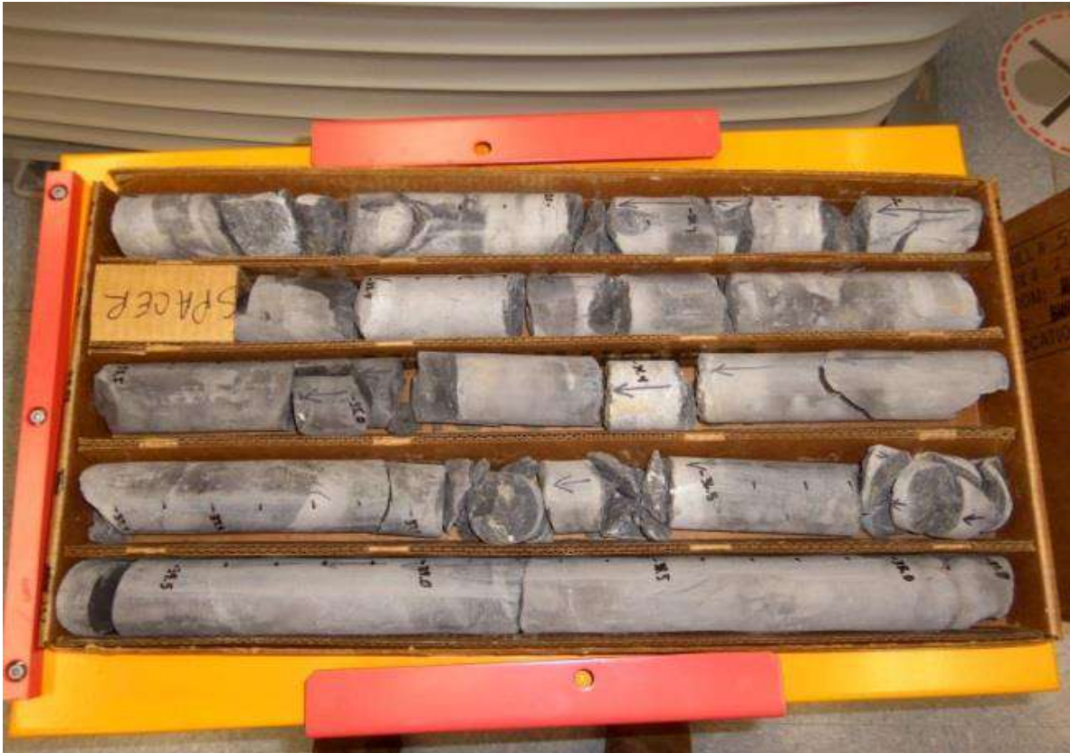
Figure 8-14. Photograph of a box of Lost River core. Note color variations (light gray to gray) that suggest relatively high carbonate and low organic content in this sampling of the Martinsburg Formation. (Image: U.S. DOE).
