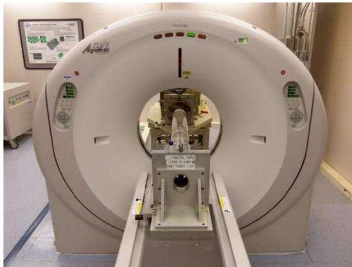
Figure 8-8. A 16-slice Aquillion medical CT scanner, similar to the unit in use at NETL.
