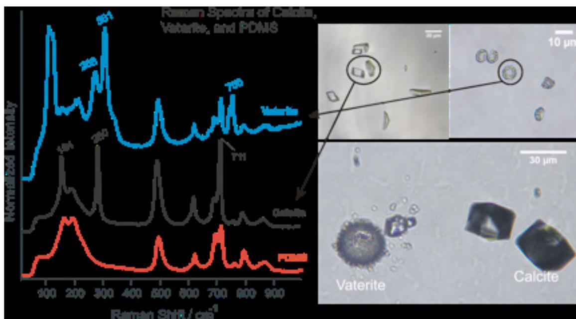
Figure 3: Raman spectra of calcite, vaterite, and PDMS. (a) Illustrates calcite crystals grown from  $\text{CaCl}_2$ . (b) Illustrates vaterite crystals grown from  $\text{CaCl}_2$  with L-aspartic acid. (c) Illustrates structures of calcite and vaterite crystals grown on the same PDMS membrane. The raman spectra to the left shows distinct peaks specific to crystalline calcium carbonate polymorphs, vaterite and calcite, as well as those for the PDMS substrate.
