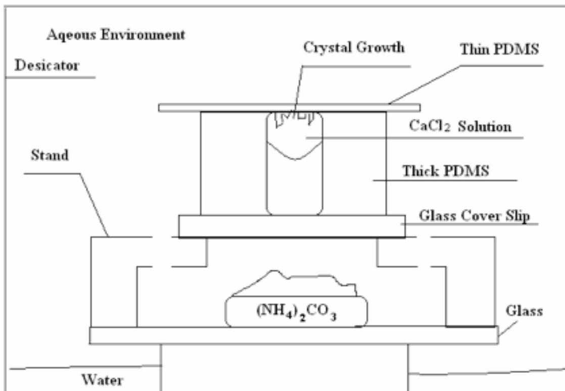
Figure 1: Experimental set up for production of calcite crystals.
