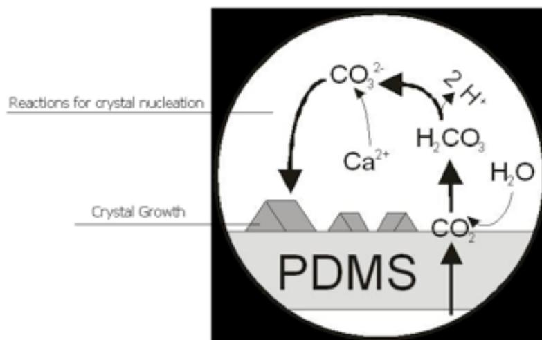
Figure 2, above: Illustrates how the ions of Ca<sup>+2</sup> and CO<sub>3</sub><sup>2-</sup> combine to form calcium carbonate crystals.
