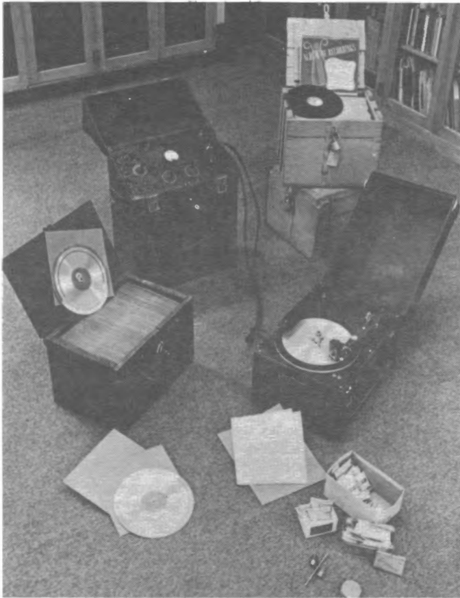
Chappell employed this handmade recording machine in recording over two thousand folksongs throughout West Virginia between 1937 and 1947. Photo by Carl Fleischhauer.
