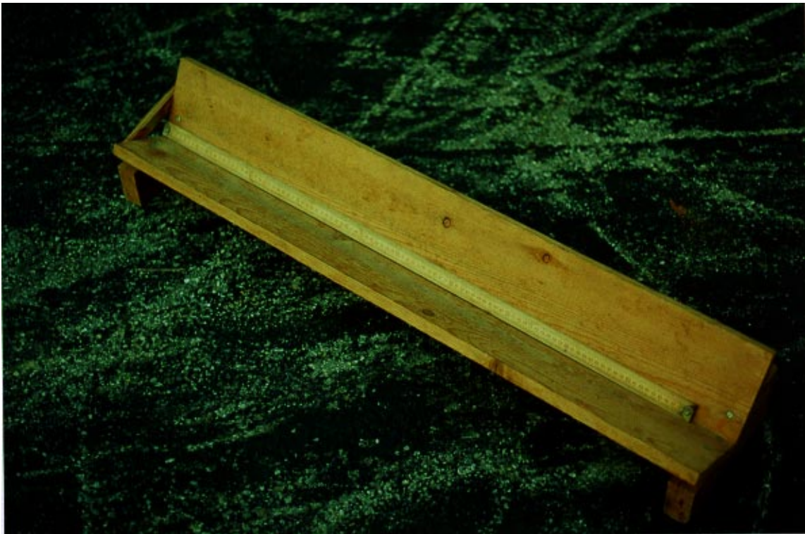
Figure 19. Measuring trough used to determine the length and diameter of fruit at harvest.
