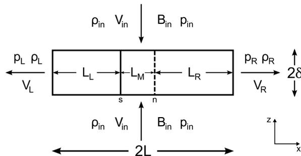
**Figure 1.** Sweet-Parker-like reconnection with asymmetric downstream pressure and a pressure gradient through the current sheet. The solid vertical bar inside the current sheet (marked  $s$ ) represents the flow stagnation point and the dashed vertical bar (marked  $n$ ) represents the magnetic field null.
