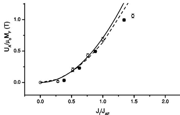
FIG. 6. Normalized effective anisotropy energy generated by the interface interaction as a function of the interface exchange energy  $J_{I1}=J_{I2}\equiv J_I$  ( $\circ$ ) and  $J_{I1}-J_{I2}=5.0$  K, with  $(J_{I1}+J_{I2})/2\equiv J_I$  ( $\bullet$ ). The continuous line corresponds to Slonczewski's model with  $M_F=M_{AF}=1$  and the dashed line to the same model but using the Monte Carlo-computed values of  $M_F$  and  $M_{AF}$ .
