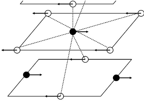
FIG. 1. Representation of the cells used for the simulations. The axes are indicated in the figure. The  $\circ$  and  $\bullet$  represent the two AF magnetic sublattices and the dotted lines indicate the nearest-neighbors. The magnetic spin ordering corresponds to the bulk AF at low  $T$ .
