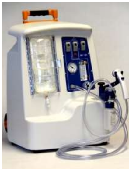
Figure 5. Microbial wet-vacuum DNA collection system, alternatively referred to as the M-VAC ® [72].
