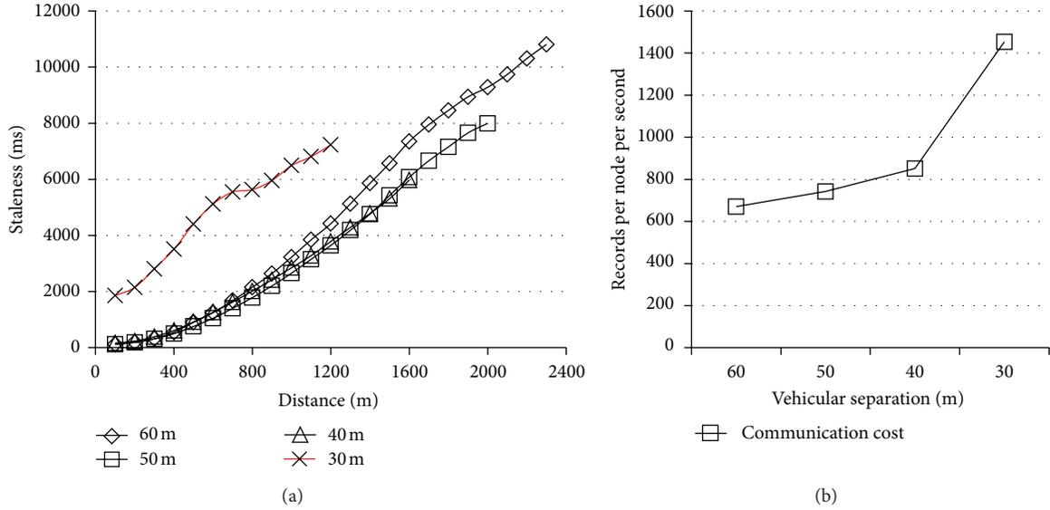
FIGURE 8: Impact of network density on VCAST: (a) maximum staleness versus pairwise vehicular distance with 784 vehicles, Communication range 100 m, source broadcast rat 10 Hz, separation 60 m, 50 m, 40 m, and 30 m. (b) Number of vehicular records transmitted by each node per second with 784 vehicles, communication range 100 m, source broadcast rat 10 Hz, separation 60 m, 50 m, 40 m, and 30 m.
