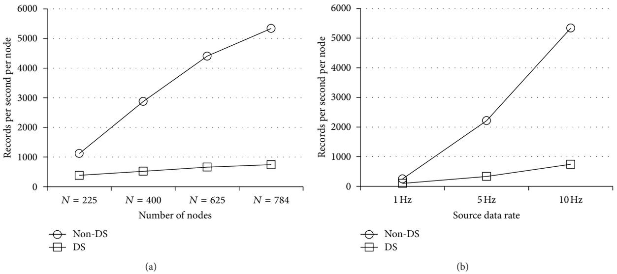
FIGURE 5: Comparison of message complexity: VCAST versus non-distance-sensitive forwarding. (a) Number of vehicular records transmitted per second per node at different network sizes for  $p = 10$  Hz and range 100 m. (b) Number of vehicular records transmitted per second per node at different source broadcast rates for 784 nodes and range 100 m.
