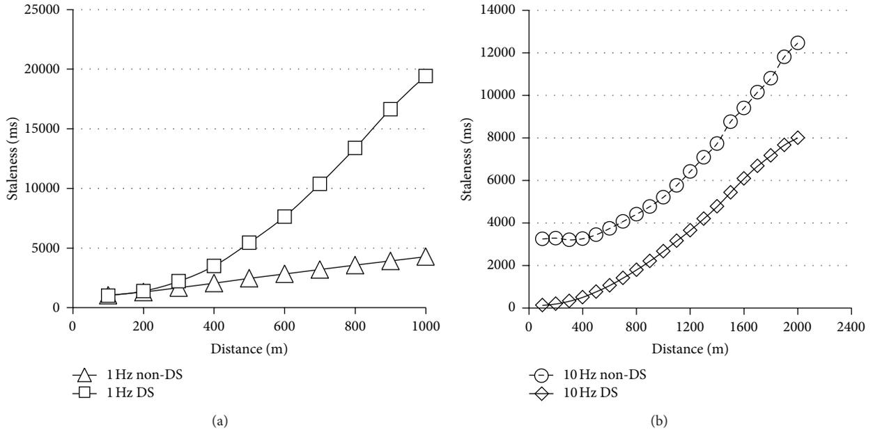
FIGURE 4: Impact of source broadcast rate: VCAST versus non-distance-sensitive forwarding. (a) Maximum staleness versus pairwise vehicular distance:  $p = 1$  Hz at 784 nodes. (b) Maximum staleness versus pairwise vehicular distance:  $p = 10$  Hz at 784 nodes.
