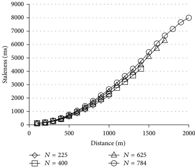
FIGURE 3: Maximum staleness versus pairwise vehicular distance for VCAST:  $p = 10$  Hz, network sizes of 225, 400, 625 and 784 vehicles, communication range 100 m, separation 50 m. Staleness values are preserved at corresponding intervehicular distances, irrespective of network size.
