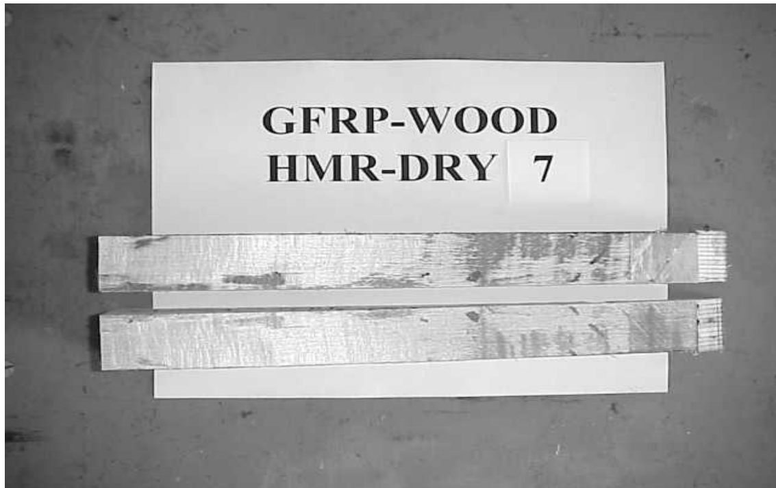
Figure 5.28. Fractured faces of Epoxy FRP-wood/HMR/dry specimen (HMR-DRY 7)
