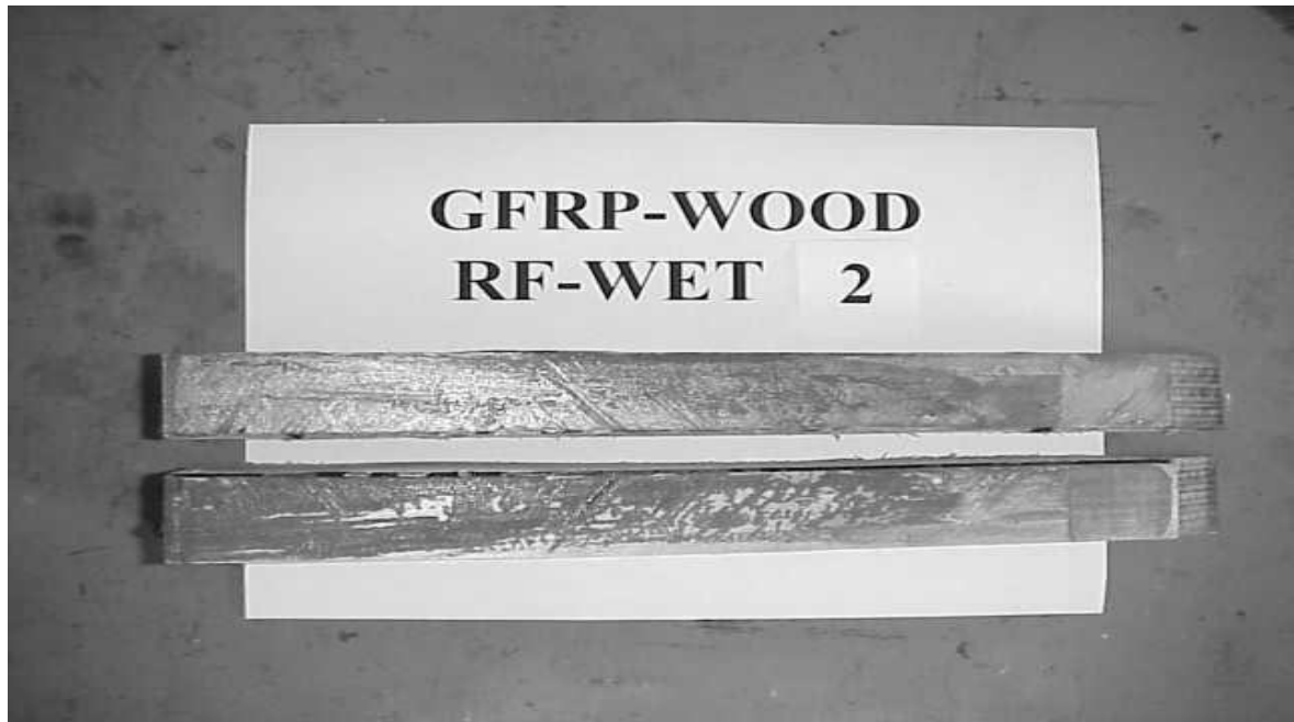
Figure 5.34. Fractured faces of Epoxy FRP-wood/RF/wet specimen (RF-WET 2)
