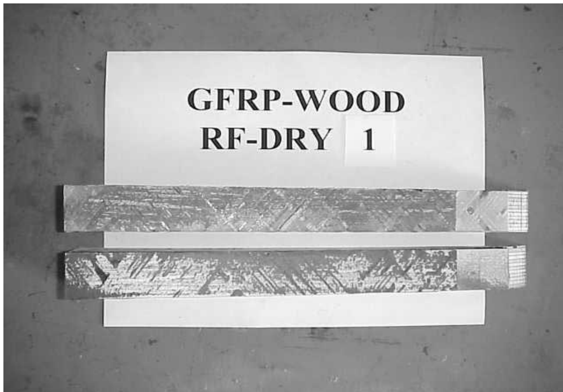
Figure 5.30. Fractured faces of Epoxy FRP-wood/RF/dry specimen (RF-DRY 1)
