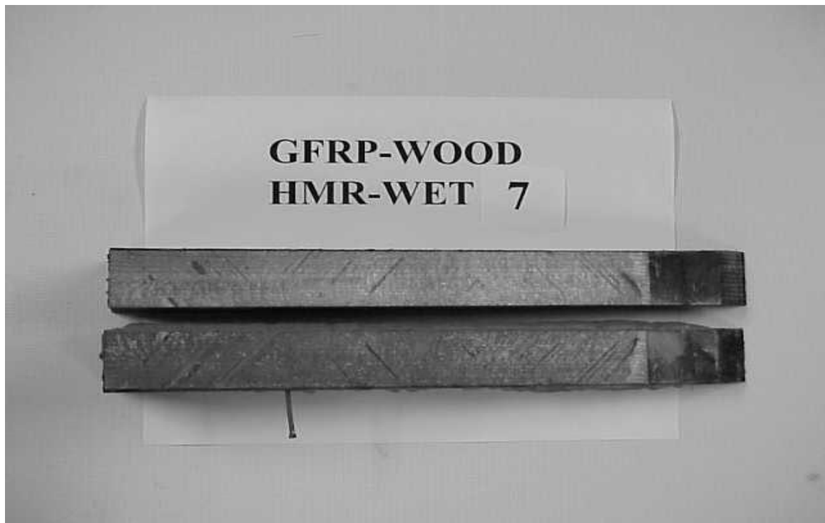
Figure 5.32. Fractured faces of Epoxy FRP-wood/HMR/wet specimen (HMR-WET 7)
