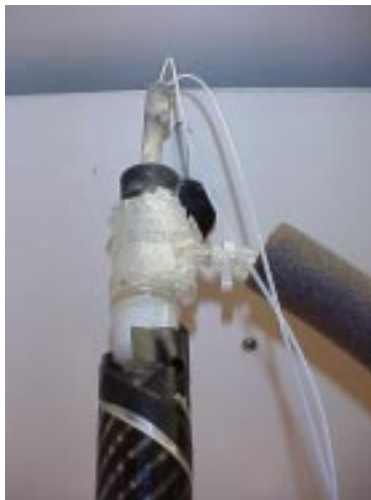
Figure 3-4. Custom distillation head inserted into top of packed column.
