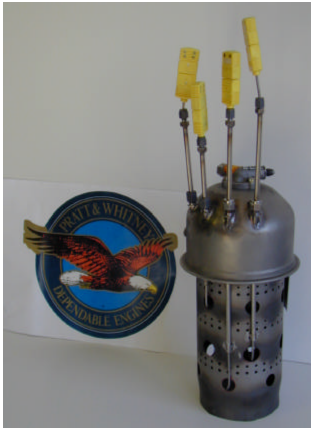
Figure 4.1 - Photographs of Thermocouple Equipped Combustor Can as Modified by WVU and Pratt and Whitney Canada
