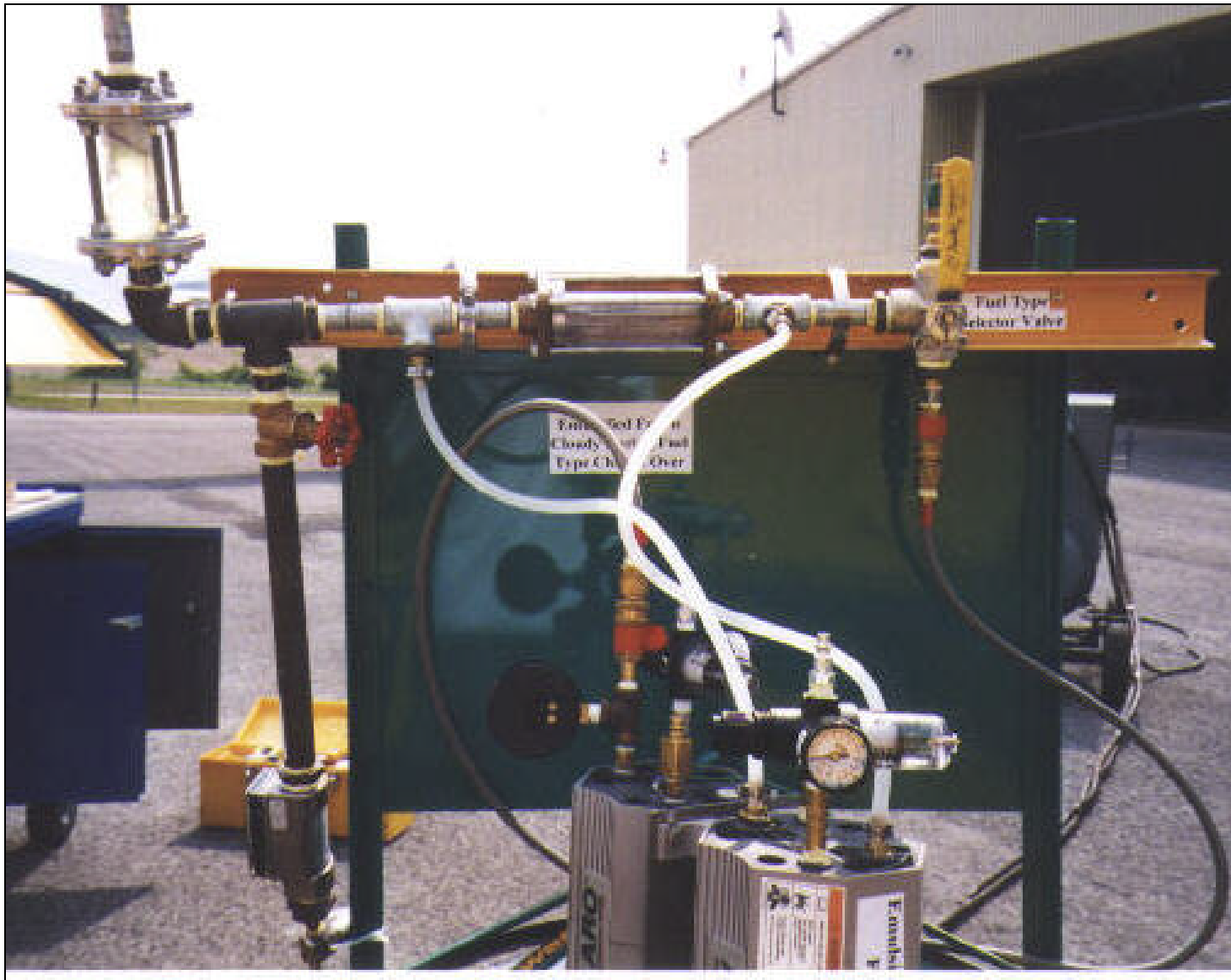
Figure 2.9 - Fuel Selector and Emulsifier
