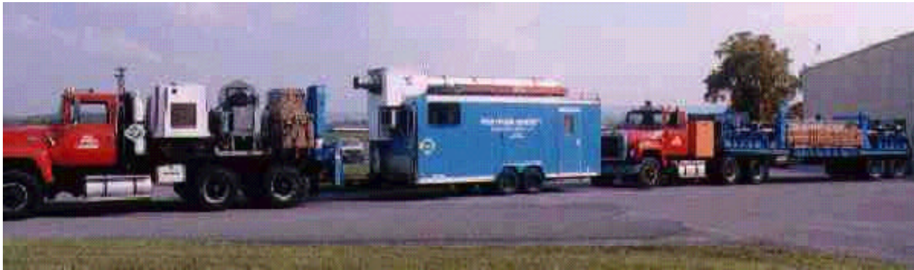
Figure 6.1 - WVU mobile emissions lab and mobile testing equipment
