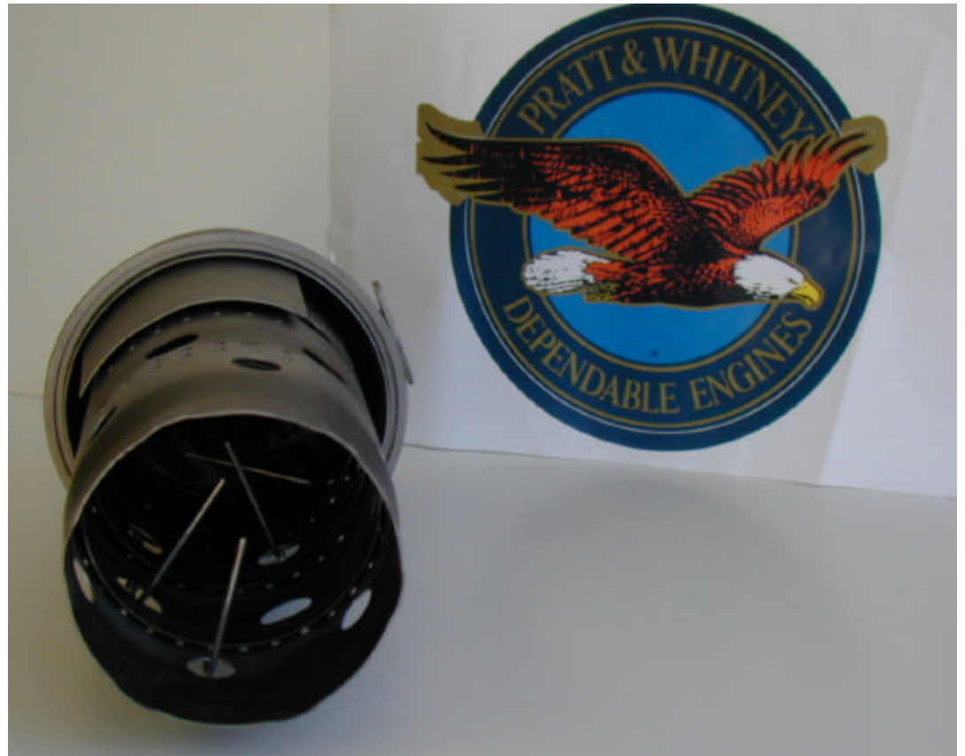
Figure 4.1 - Photographs of Thermocouple Equipped Combustor Can as Modified by WVU and Pratt and Whitney Canada
