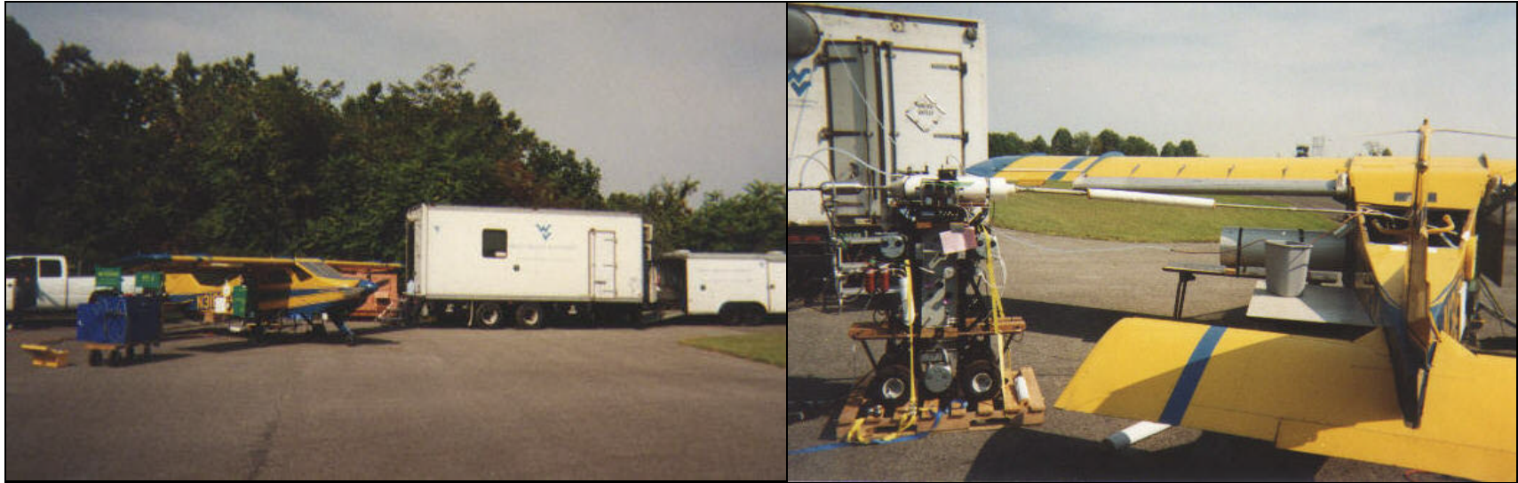
Figure 6.2- WVU mobile emissions lab and STOL research aircraft setup for engine testing
