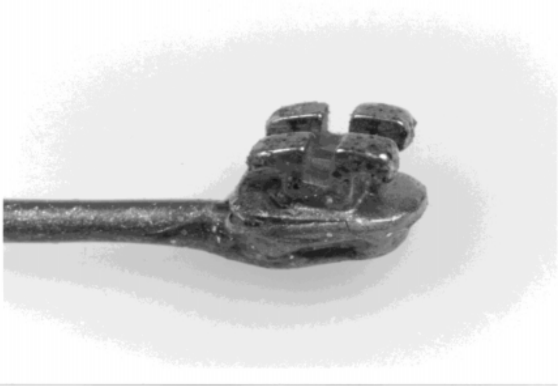
Figure 4. Stainless steel bracket after testing
