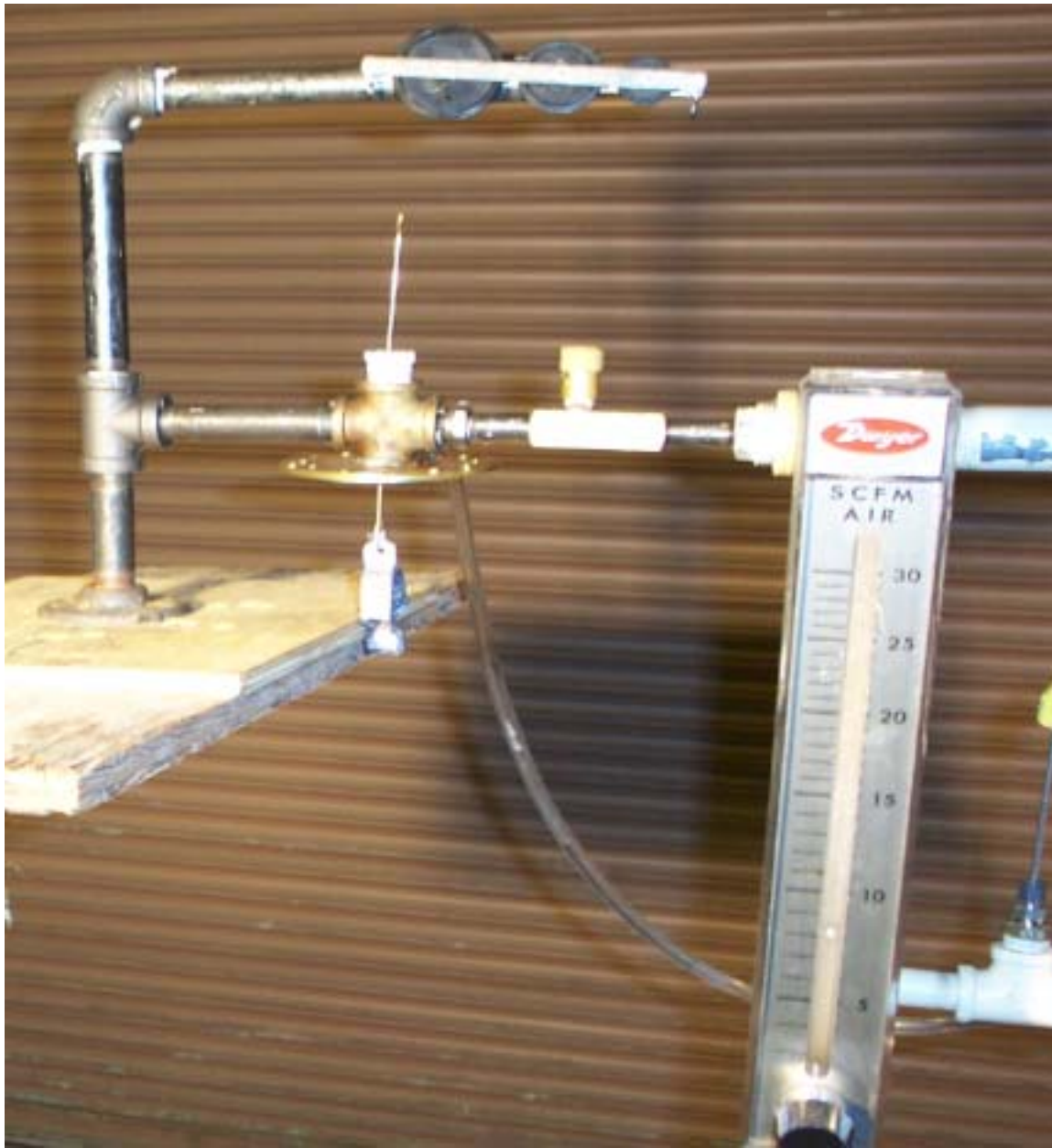
Fig 5.6: Picture of Diaphragm Suspended by Air Flow with a Weight of 43.5 Grams
