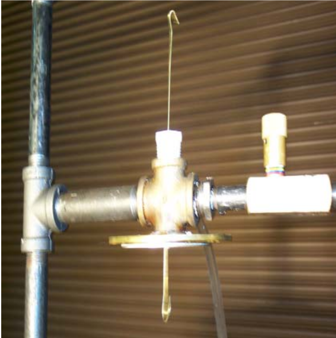
Fig 5.7: Picture of Diaphragm with its Own Weight of 21 Grams Suspended by Air Flow.
