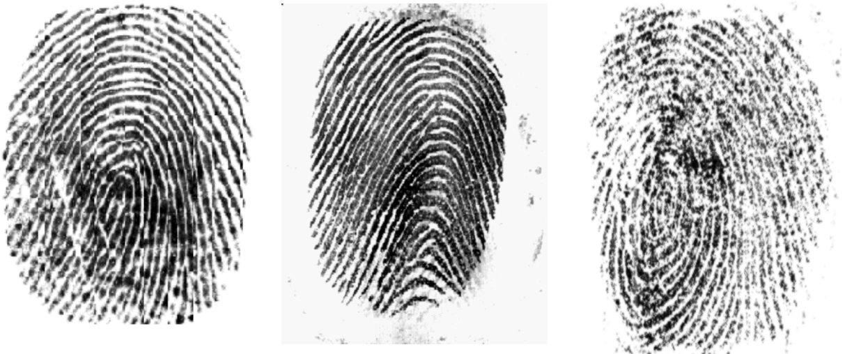
Figure 1.1: Images captured with commercial fingerprint sensors from live, cadaver and spoof fingers.
