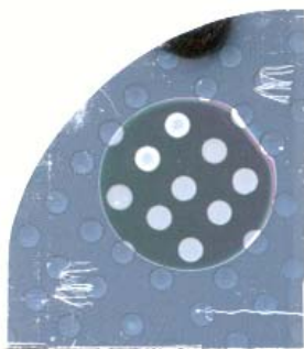
Figure 2-13: A typical sample for CV measurements. Small circular pads are aluminum top contacts.
