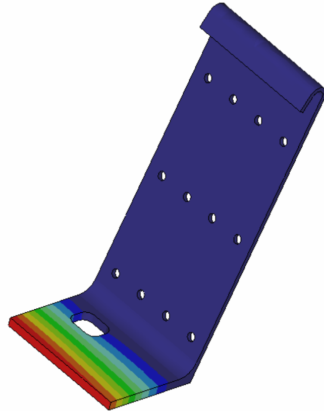
Figure 45: Analysis of Pod Attachment Bracket in the Stowed Position
