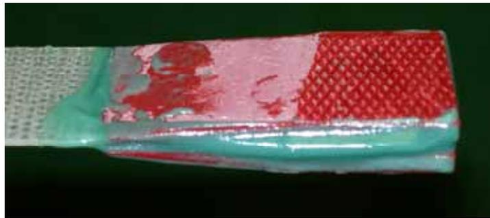
Figure 3. Reinforcement tabs after application to sample - side view
