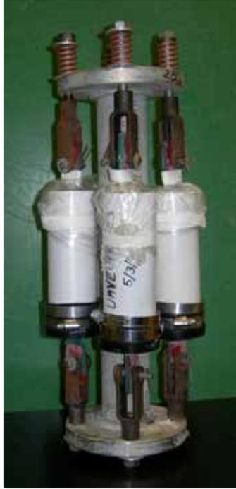
Figure 2. Sustained load test assembly
