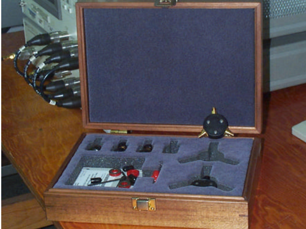
E.10 The calibration kit used to calibrate the network analyzer.
