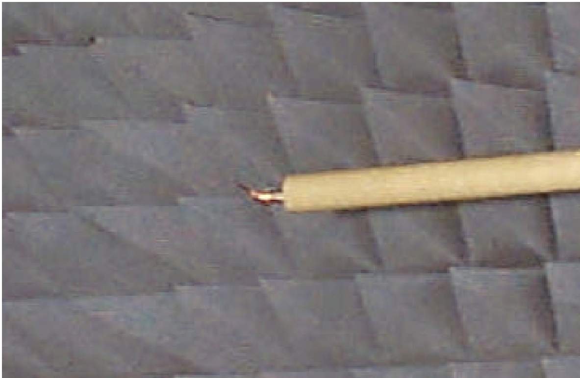
E.7 The transmitting dipole mounted horizontally
