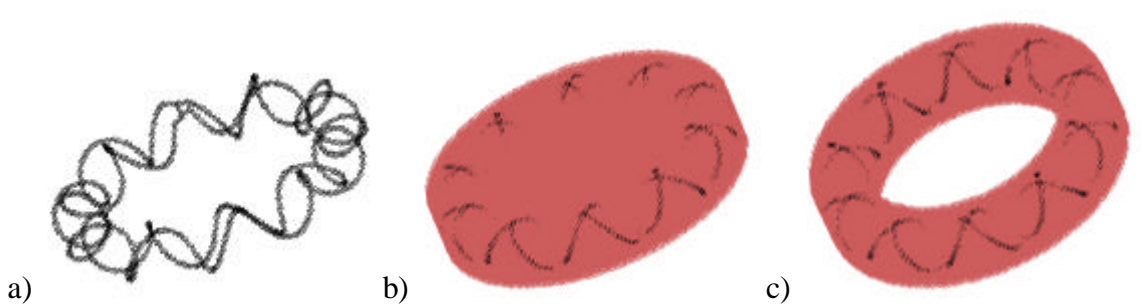
Figure 2.1 The core CTHA: a) wire only, b) full core, c) hollow core
