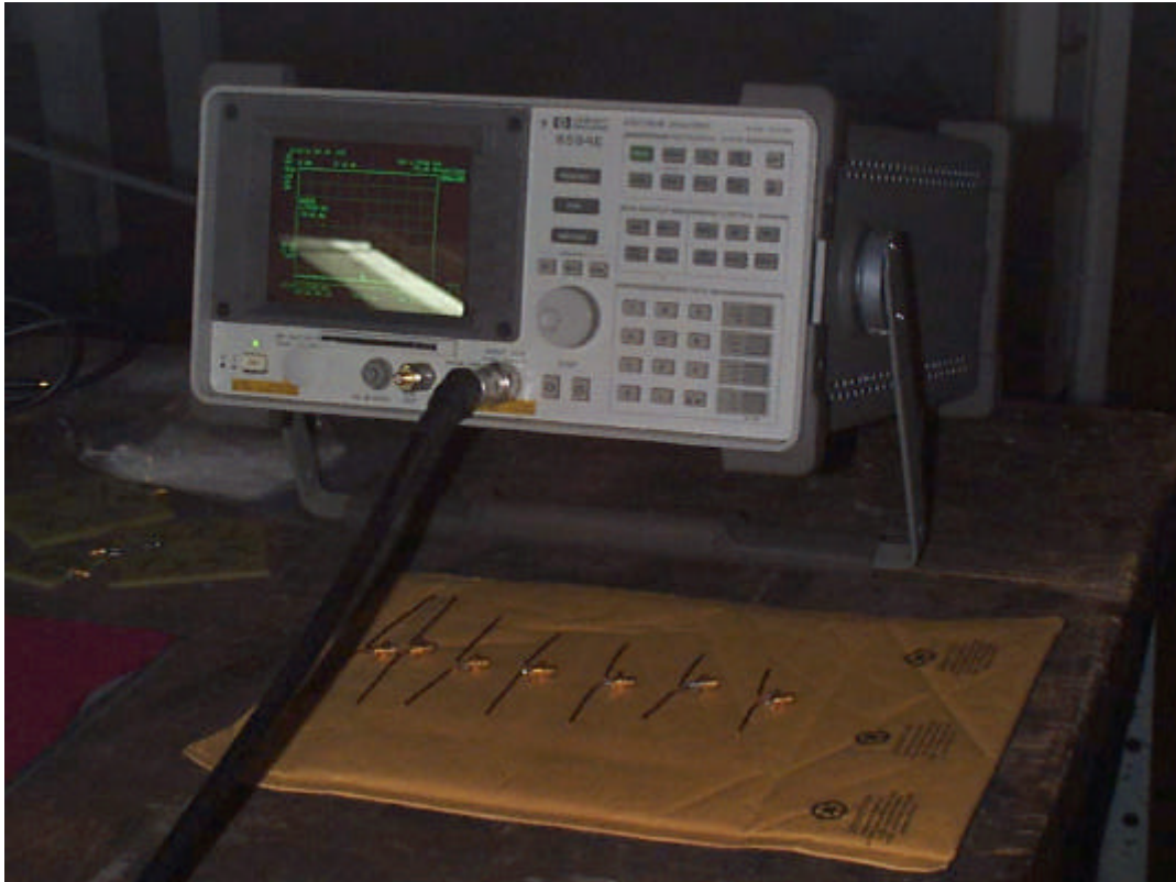
E.13 The Spectrum Analyzer, with the dipoles used for the experimental analysis shown.
