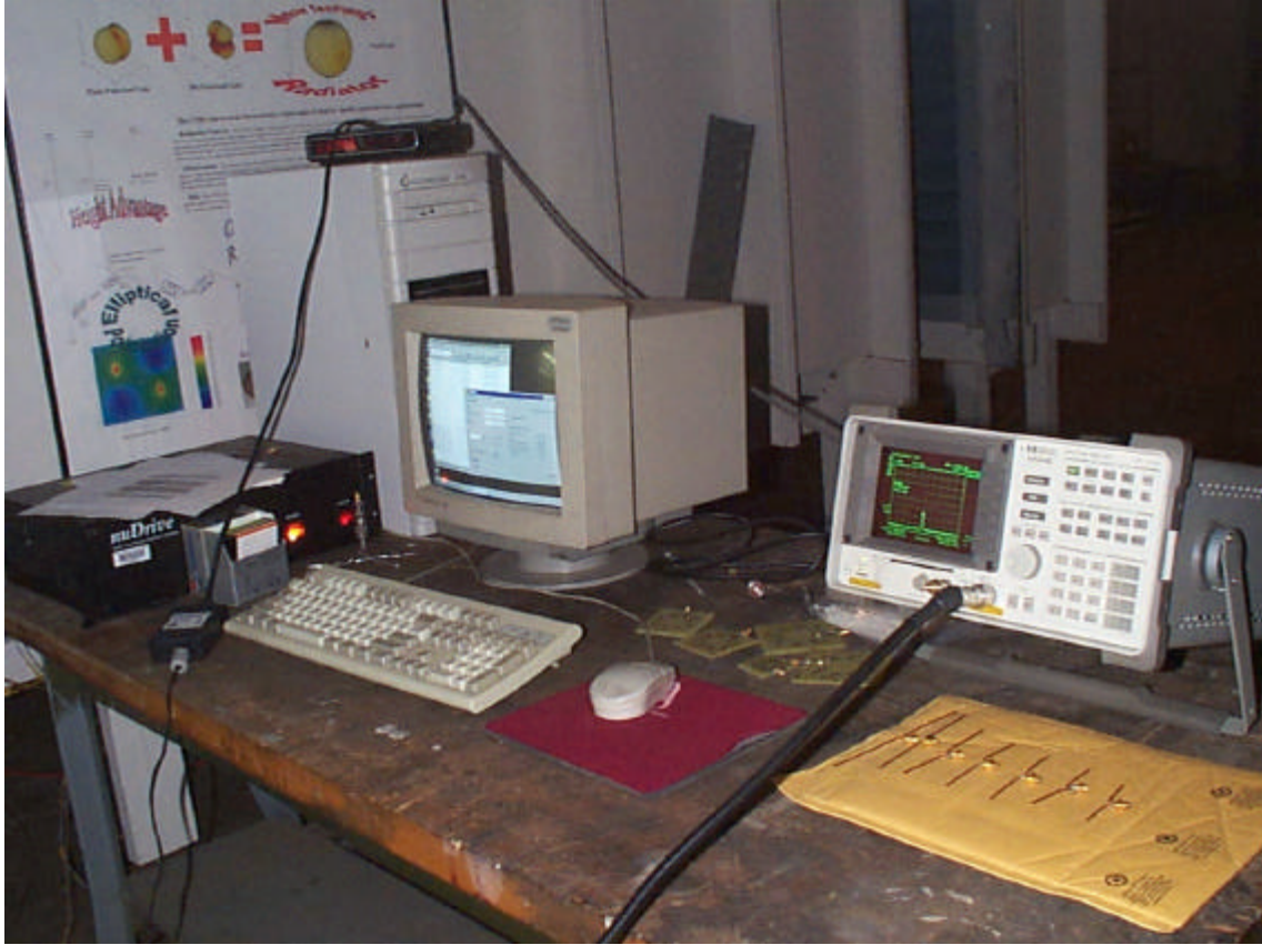
E14 The experimental workbench, with the computer, rotator motor, the spectrum analyzer, the CTHAs, and the dipoles visible. The anechoic chamber is also partially visible behind the workbench.
