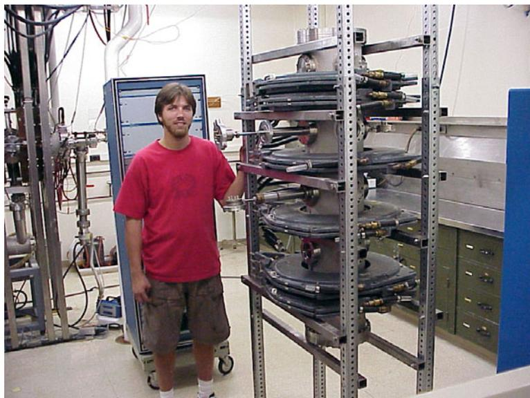
**Figure 2.** Photograph of the vertical Q machine during construction, with graduate student Eric Reynolds. Some probes are attached to the chamber. Magnet power, cooling water and plasma sources are not yet installed.
