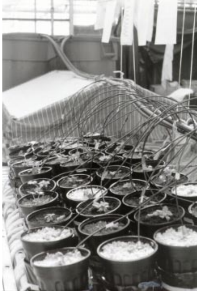
Figure 4-1: Nutriculture bench set-up for production of individual Fragaria x ananassa cv. 'Fresca' plants with effluent collection tubes for individual pots and drip emitters for irrigation from the stock tanks in the background.
