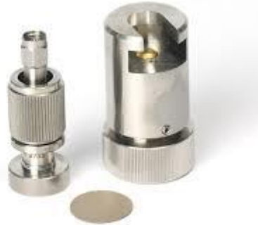
Figure 2.9: Standard Keysight High Temperature Coaxial Probe, used to collect scattering parameters from a material so a VNA can calculate the material properties 36 .
