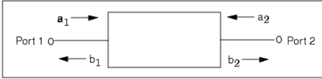
Figure 2.5: Single wave in a two-port electrical-element. Simple representation of a standard 2 port measurement for S-parameters 32 .
