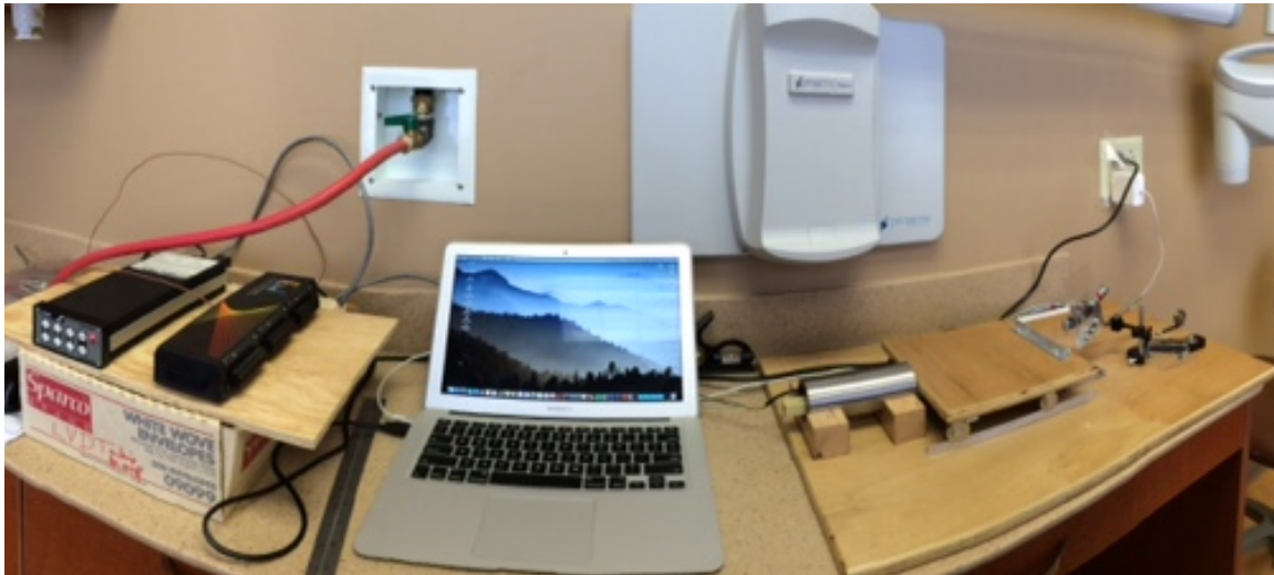
Figure 2. Experiment Assembly From left to right: LVDT signal conditioner, Personal Daq/3000, laptop used to run Daq/3000 software, experiment apparatus.
